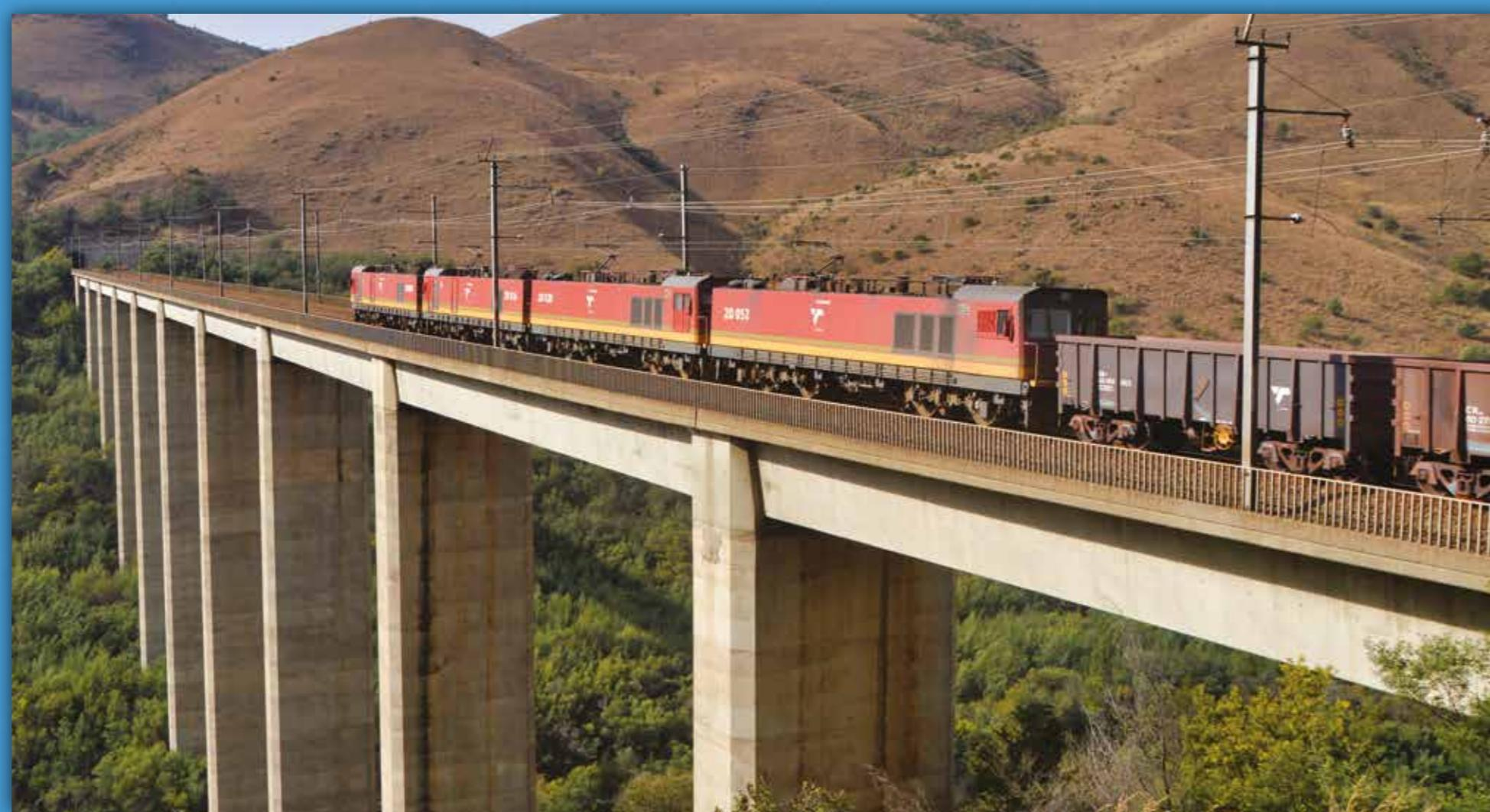
Class 20E's 20-006, 20-014, 20-020 and 20-052 make light work of a load of empty CR wagons as they climb Majuba Pass heading to tunnel #3 while crossing bridge #3 with its 11X45m spans 77m above the Harte River on 15 July 2017. Photo: Brandon M. Stow
