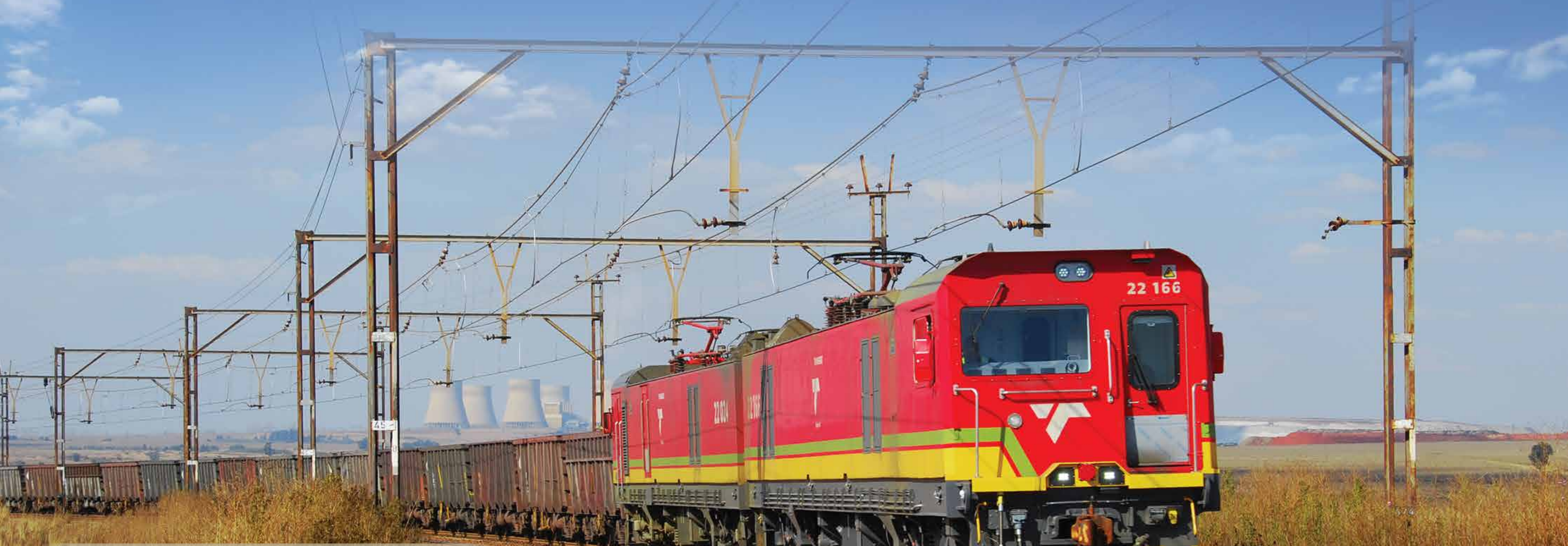
The Class 22E single cab dual voltage electric locomotive fleet is being built by the Zhuzhou Electric Locomotive Company, a subsidiary of CRRC Corporation Ltd, principally a Chinese state owned enterprise. The first 40 locomotives were fully imported while the remainder of the fleet, eventually to comprise 359 locomotives, is being built locally at Transnet Engineering's Koedoespoort Works in Pretoria. Here locally built 22166 leads China built 22024 with a load of empty ore wagons west-bound between Arbor and Argent in Mpumalanga Province on Saturday afternoon 26 May 2018. Eskom's Kendal Power Station looms in the background. The catenary shows evidence of a third track on the right, now removed, installed in steam days on the long climb between Arbor and Argent to expedite coal traffic from Witbank to the Reef and beyond. Photo Peter A. Stow
