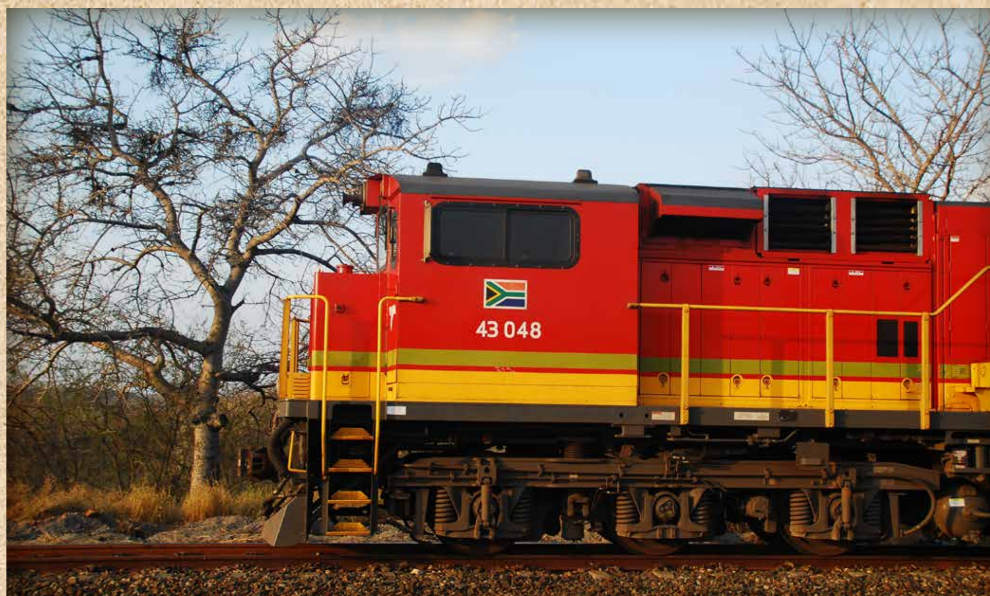
Transnet is understandably "Proudly South African" with the Transnet Engineering assembled General Electric class 43 diesel electric locomotives. The Graham-White 994 air dryer, represented in South Africa by Vanrail, can be clearly seen below the sidesill between the locomotive bogies. Photo: Brandon M. Stow
